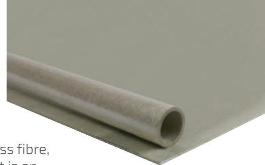
Mikla 990's low thermal conductivity allows saving energy costs substantially. As a result of low water absorption and chemical stability, there is an increase in the life expectancy of this material. It consists of glass fabric, glass fibre, glass mat and mica paper, as well as to high temperatures resistant resins. It is an asbestos-free product, resistant to high temperatures and has a good mechanical resistance even at high temperatures.
